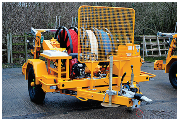
Puller for distribution lines
