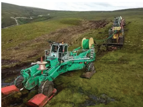
Laying system in mud and bog areas
